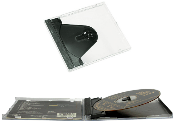
The original MFSL CD case: Patented mechanism raises the CD away from the tray when the case is open allowing you to remove the CD by the edges and locks the CD into the tray when the lid is closed.
